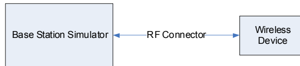
Figure 11-1 Power Measurement Setup
