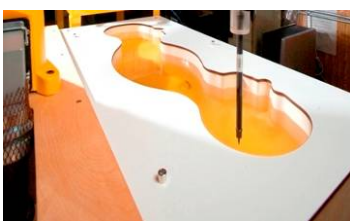
Figure 6-2 SAM Phantom with Simulating Tissue
