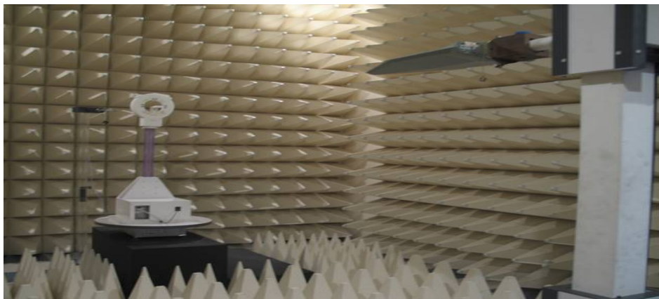
Figure2. Photograph of 3m Fully-Anechoic Chamber
