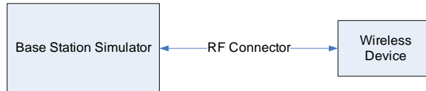
Figure 8-2 Power Measurement Setup
