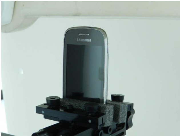
Top Side, Test Separation 1.0 cm
