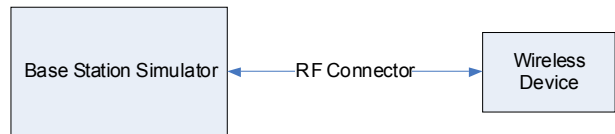
Figure 8-1 Power Measurement Setup
