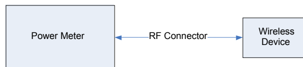
Figure 8-3 Power Measurement Setup
