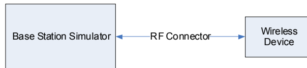
Figure 8-2 Power Measurement Setup
