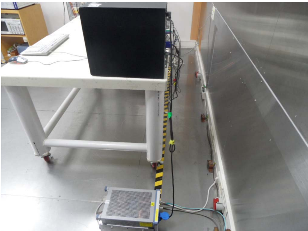
[ Conducted Disturbance – Rear ]
