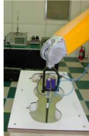
Figure 4.2 Photograph of the probe and the Phantom
