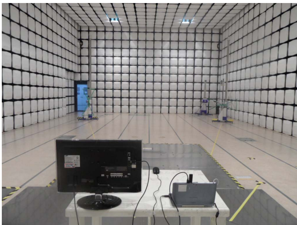
[ Radiated Disturbance for Below 1 GHz – Rear ]
