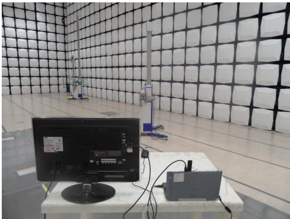
[ Radiated Disturbance for Above 1 GHz – Rear ]
