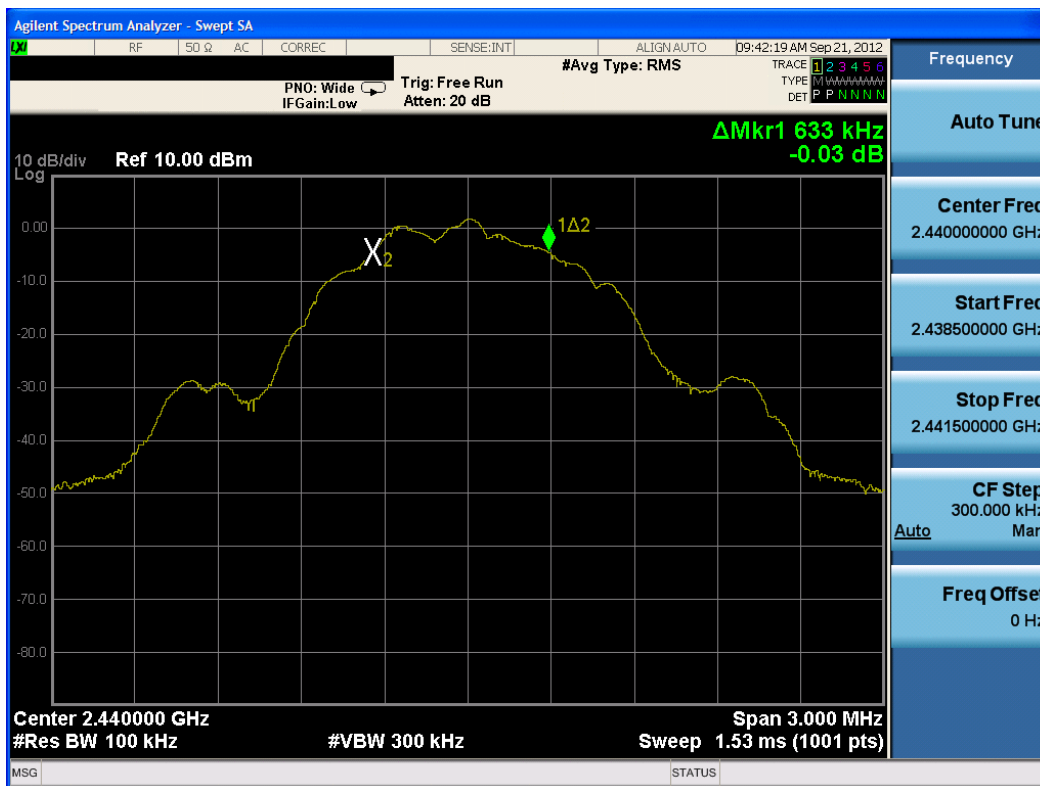
Plot 6-2. 6dB Bandwidth Plot (Bluetooth (LE) – Ch. 19)
