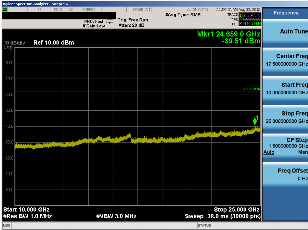
Plot 6-12. Conducted Spurious Plot (Bluetooth (LE) – Ch. 19)
