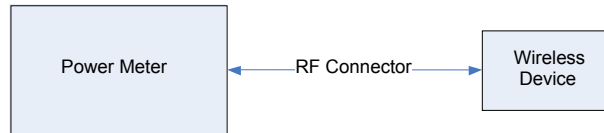
Figure 11-1 Power Measurement Setup
