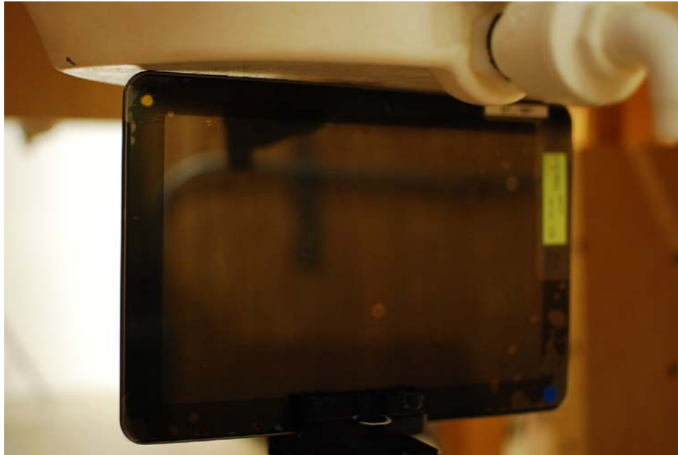
Figure 18-2 SAR Test Setup Photo 2: Top at 0.0 cm
