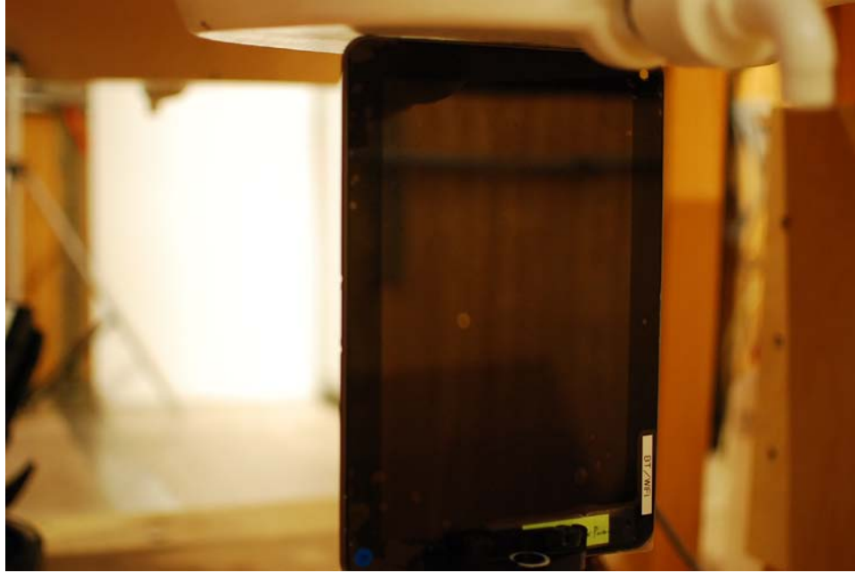
Figure 18-3 SAR Test Setup Photo 3: Left at 0.0 cm
