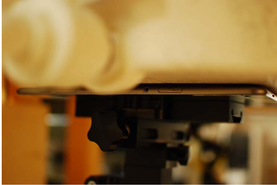
Figure 18-1 SAR Test Setup Photo 1: Back at 0.0 cm
