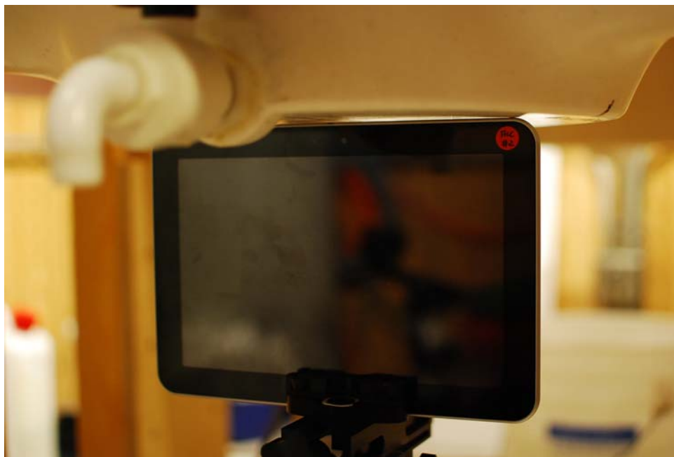
Figure 18-2 SAR Test Setup Photo 2: Top at 0.0
