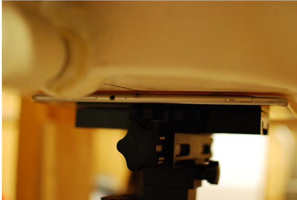
Figure 18-1 SAR Test Setup Photo 1: Back at 0.0 cm
