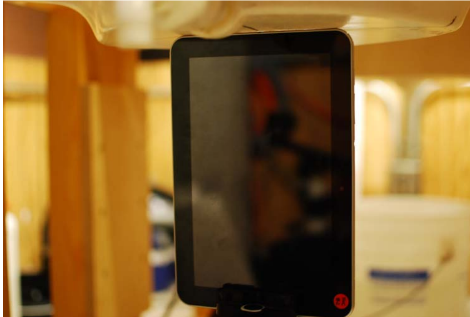
Figure 18-3 SAR Test Setup Photo 3: Left at 0.0
