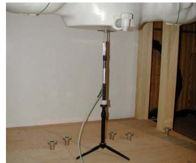
Figure 10-2 System Verification Setup Photo
