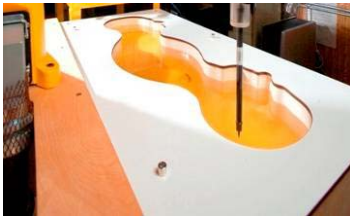
Figure 6-2 SAM Phantom with Simulating Tissue
