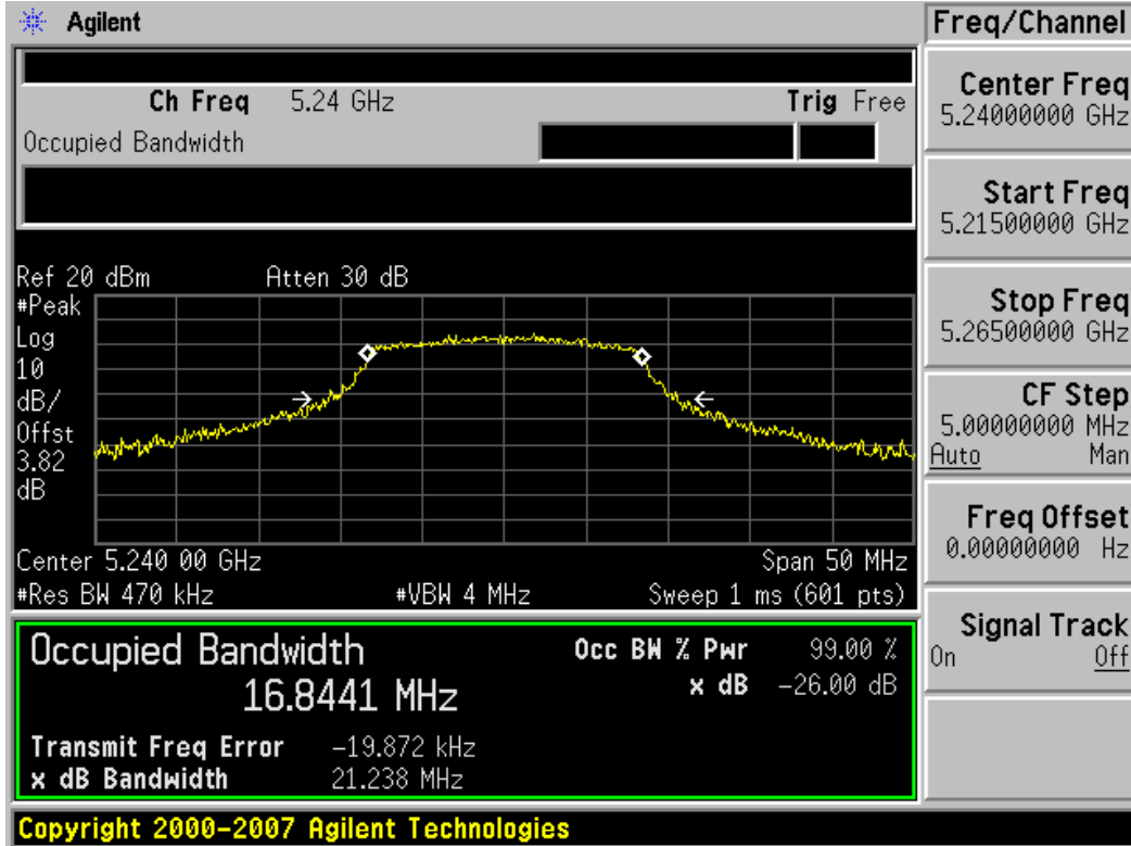
Plot 6-3. 26dB Bandwidth Plot (802.11a (UNII) – Ch. 48)
