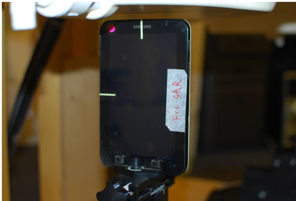
Figure 20-3 SAR Test Setup Photo 3 – Top at 0.75 cm
