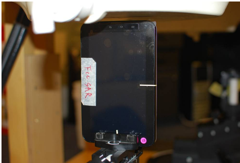
Figure 20-7 SAR Test Setup Photo 6 – Bottom at 0.5 cm
