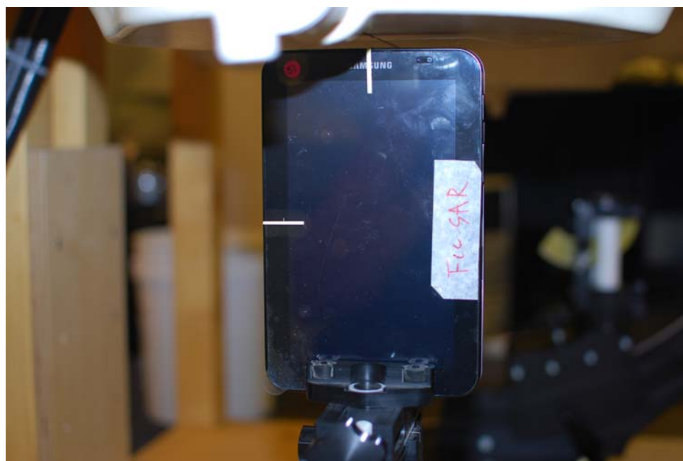
Figure 20-4 SAR Test Setup Photo 3 – Top at 0.5 cm
