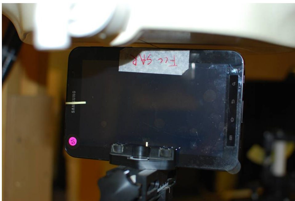
Figure 20-6 SAR Test Setup Photo 5 – Right at 0.5 cm
