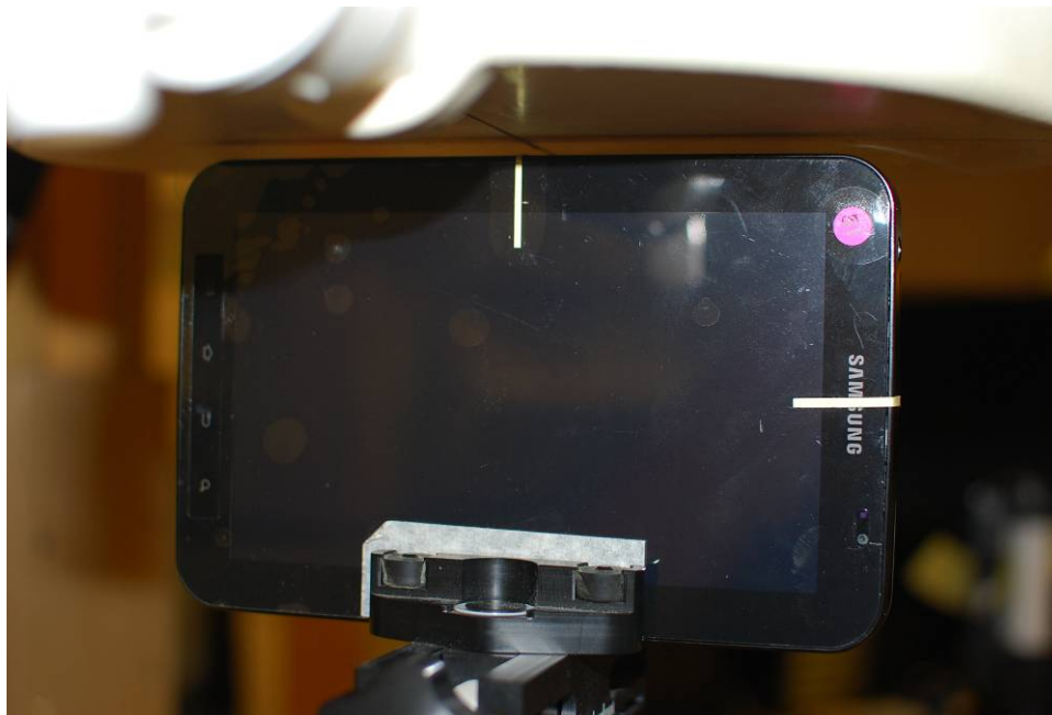
Figure 20-5 SAR Test Setup Photo 4 – Left at 0.5 cm
