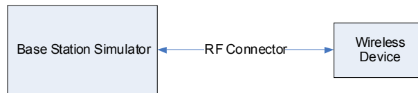
Figure 8-1 Power Measurement Setup
