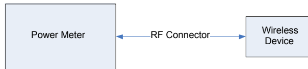
Figure 8-3 Power Measurement Setup
