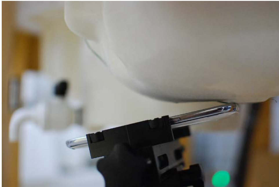
SAR Test Setup Photo 4: Left Tilt
