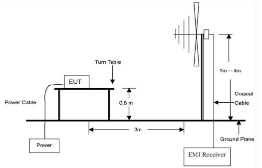
The diagram below shows the test setup that is utilized to make the measurements for emission from 1 GHz to 26.5 GHz Emissions.
