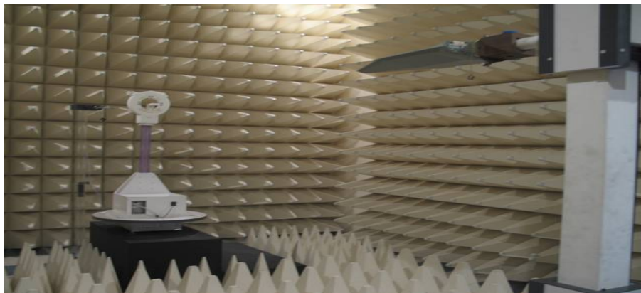
Figure2. Photograph of 3m Fully-Anechoic Chamber
