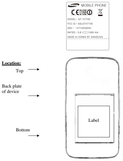
Label is placed inside of the battery compartment.
