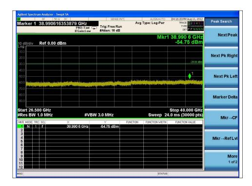
Note: Offset (d<sup>B</sup>) = Power Divider (d<sup>B</sup>) + Attenuator (d<sup>B</sup>) + Cable loss (d<sup>B</sup>) Result (d<sup>B</sup> m) = Spurious offset (d<sup>B</sup>) + Reading values (d<sup>B</sup> m)
