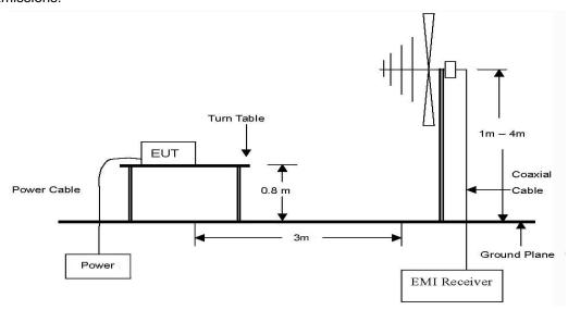
The diagram below shows the test setup that is utilized to make the measurements for emission .The spurious emissions were investigated form 1 % to the 10th harmonic of the highest fundamental frequency or 40 %, whichever is lower.
