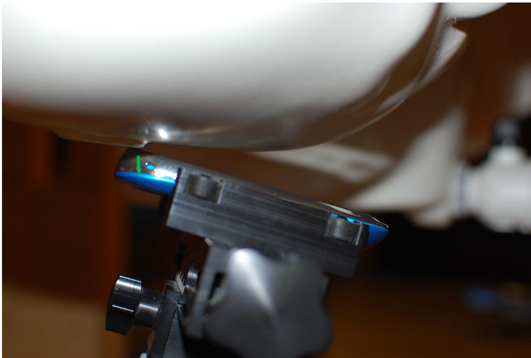
Figure 19-2 SAR Test Setup Photo 2
