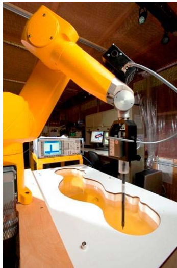
Figure 3-2 DASY4 SAR Measurement System
