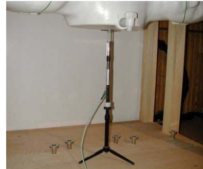
Figure 12-2 System Verification Setup Photo
