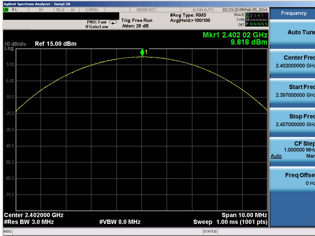
Plot 6-16. Peak Conducted Power (3Mbps – Ch. 0)
