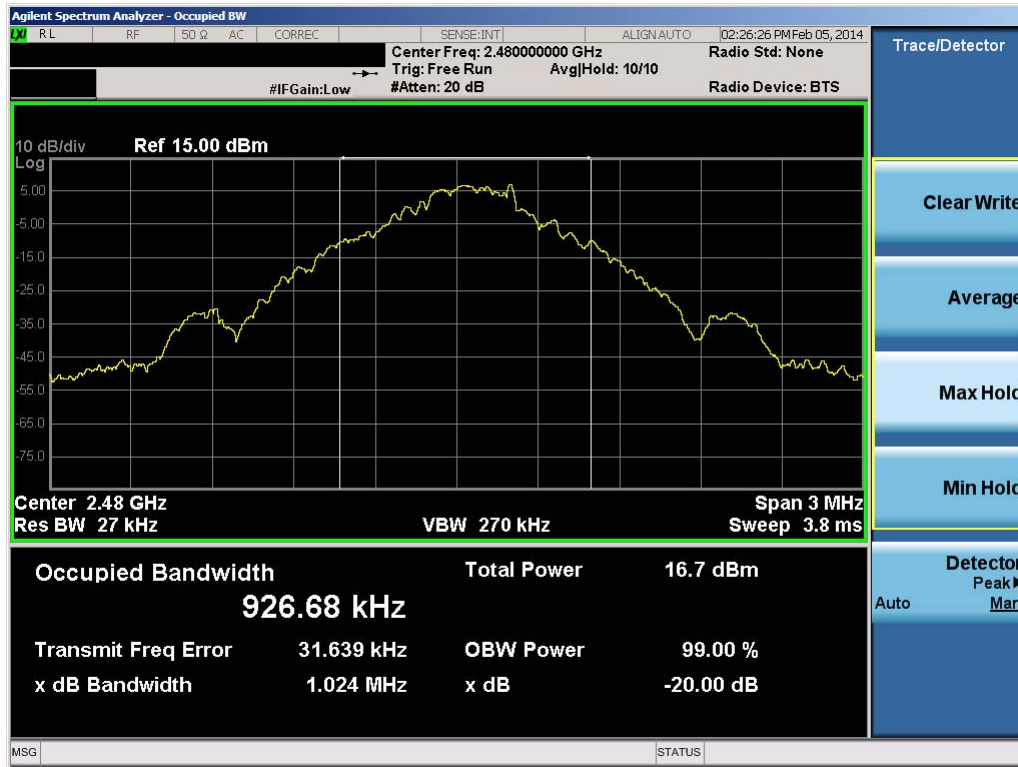
Plot 6-3. 20dB Bandwidth Plot (Bluetooth, 1Mbps – Ch. 78)
