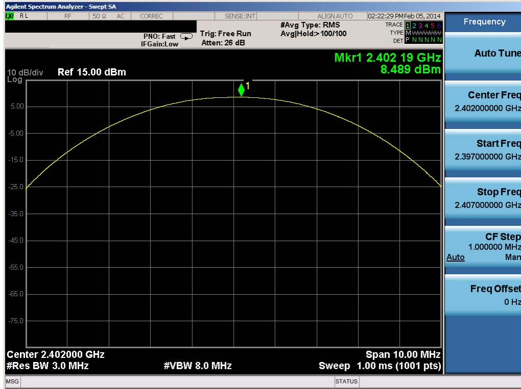
Plot 6-10. Peak Conducted Power (1Mbps – Ch. 0)
