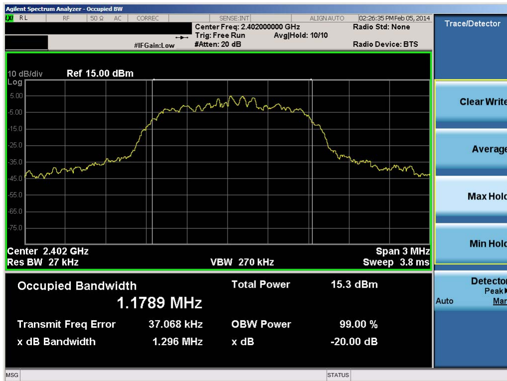
Plot 6-4. 20dB Bandwidth Plot (Bluetooth, 2Mbps – Ch. 0)
