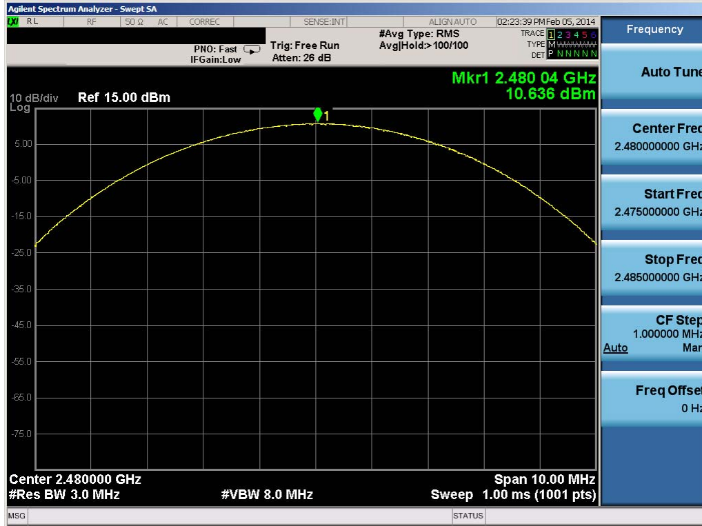
Plot 6-18. Peak Conducted Power (3Mbps – Ch. 78)
