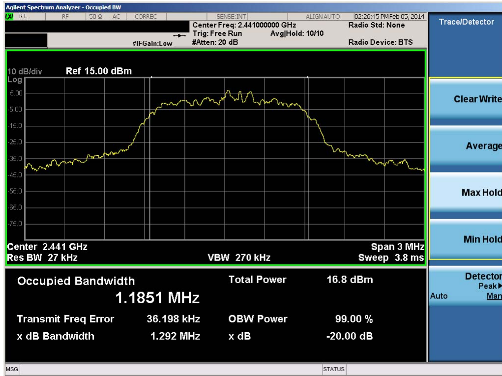
Plot 6-5. 20dB Bandwidth Plot (Bluetooth, 2Mbps – Ch. 39)
