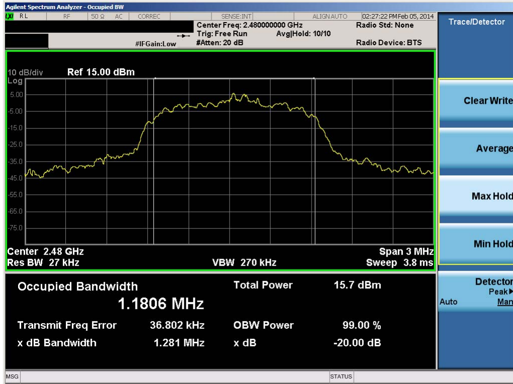
Plot 6-9. 20dB Bandwidth Plot (Bluetooth, 3Mbps – Ch. 78)
