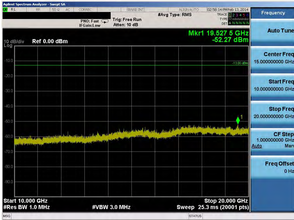
Plot 9-50. Conducted Spurious Plot (10.0MHz QPSK – RB Size 1, RB Offset 0 – Mid Channel)
