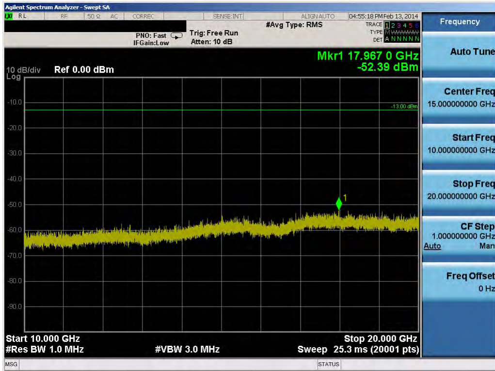
Plot 10-8. Conducted Spurious Plot (1.4MHz QPSK – RB Size 1, RB Offset 0 – Mid Channel)
