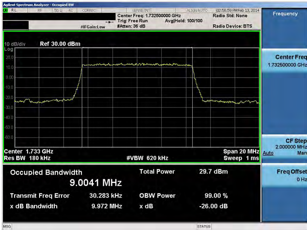
Plot 9-45. Occupied Bandwidth Plot (10.0MHz QPSK – RB Size 50)
