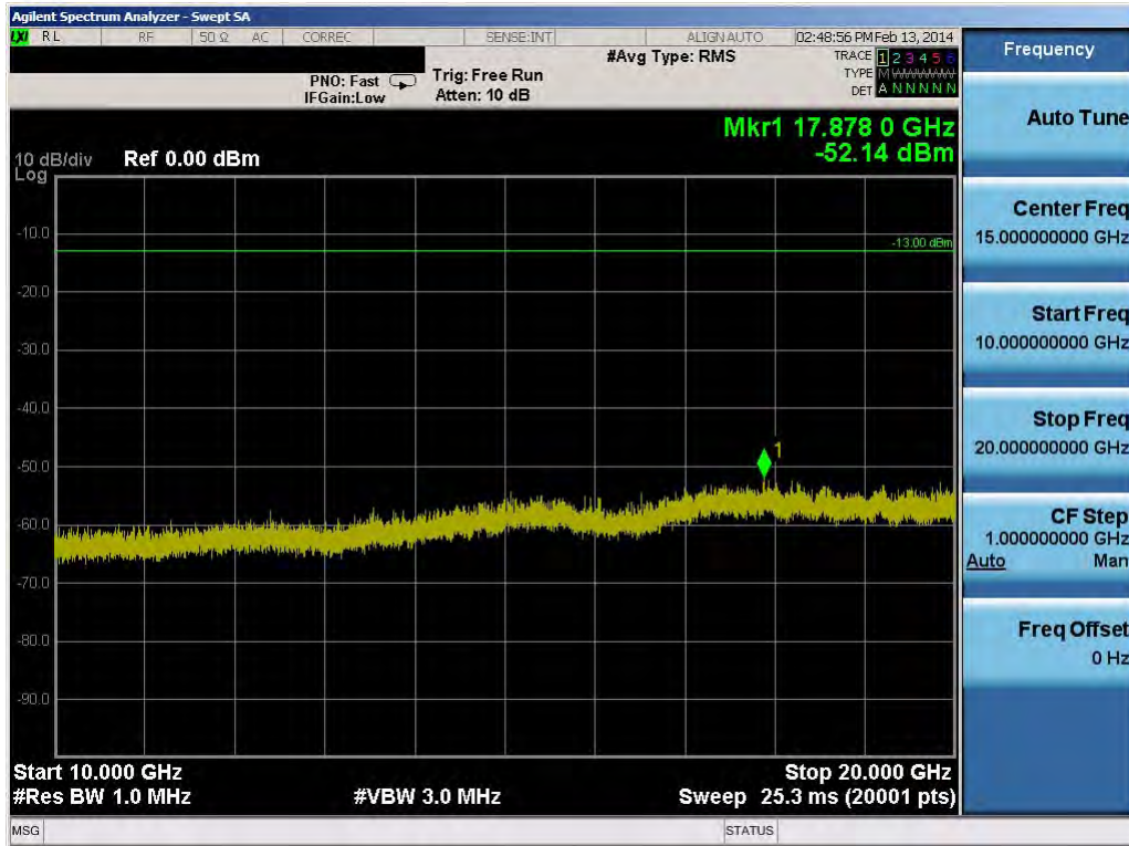
Plot 9-36. Conducted Spurious Plot (5.0MHz QPSK – RB Size 1, RB Offset 0 – Mid Channel)
