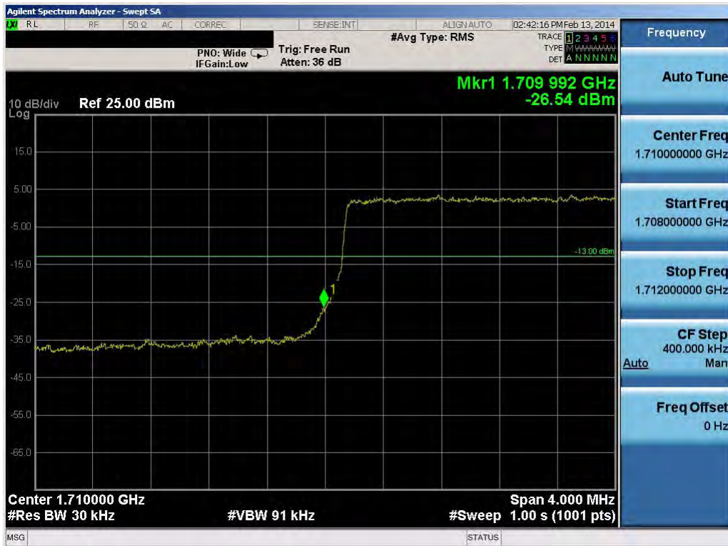
Plot 9-15. Lower Band Edge Plot (3.0MHz QPSK – RB Size 15)
