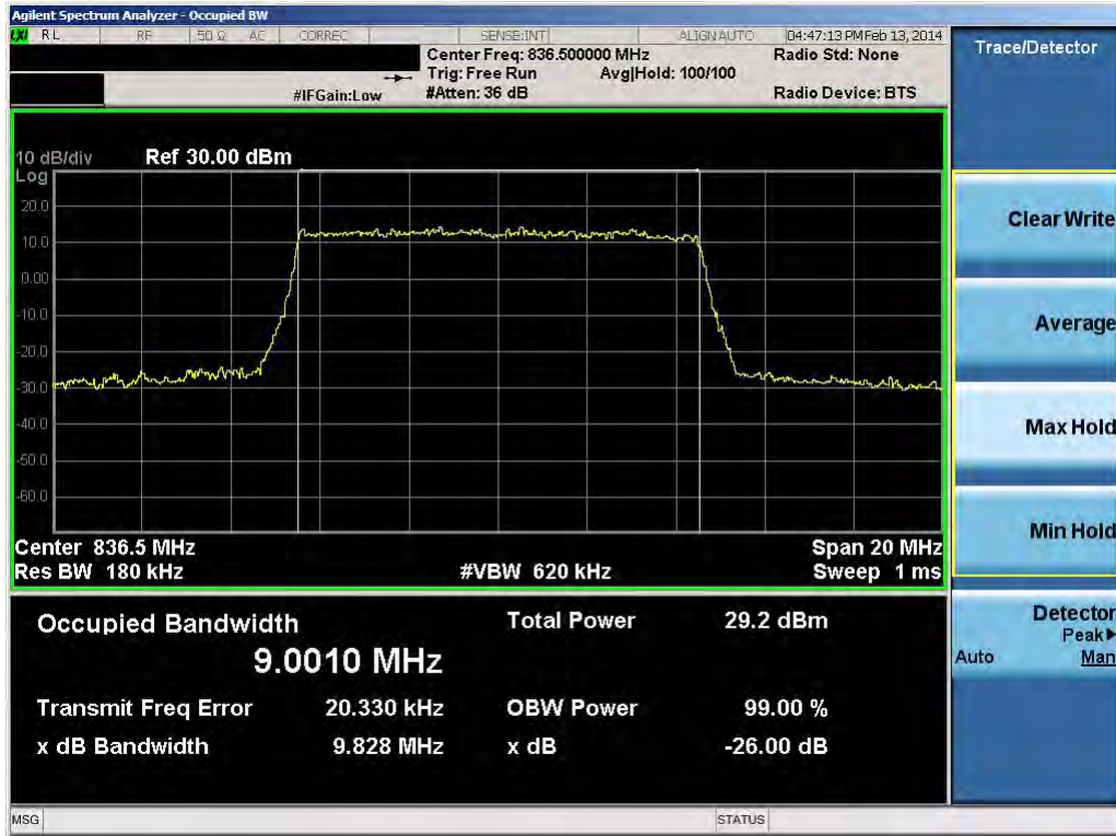
Plot 8-32. Occupied Bandwidth Plot (10.0MHz QPSK – RB Size 50)
