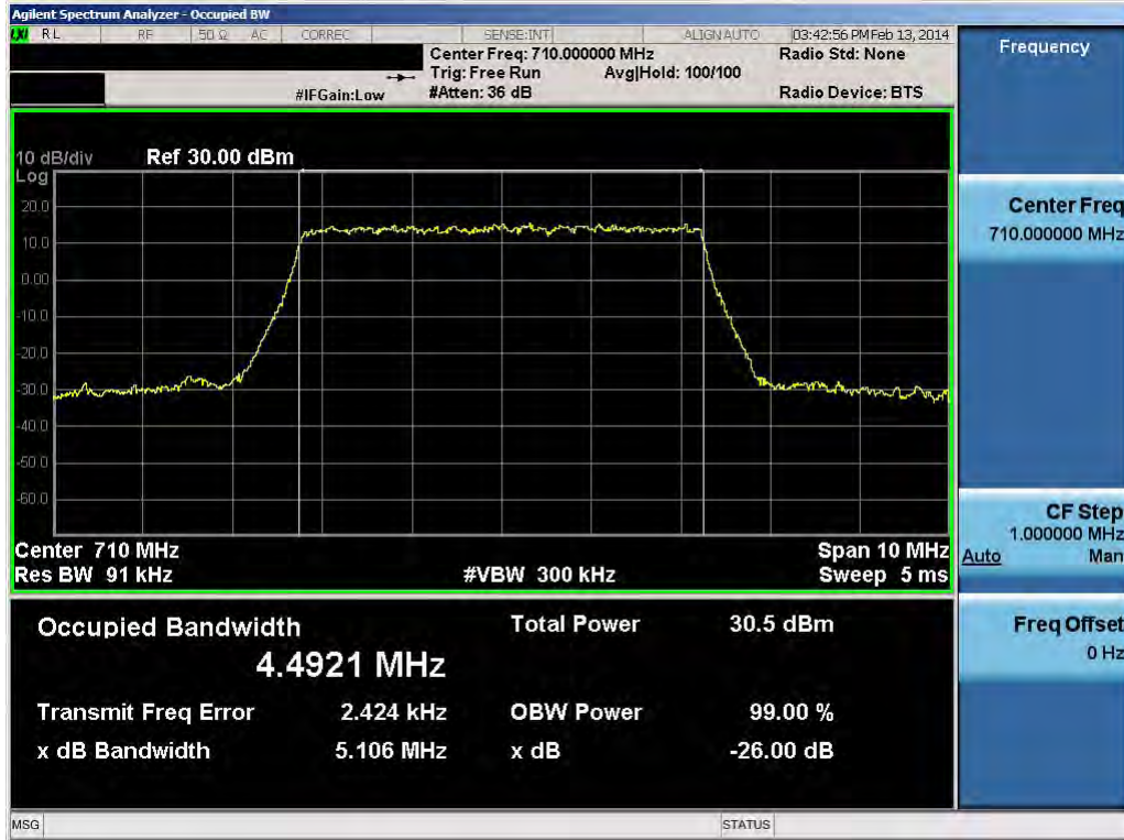
Plot 7-2. Occupied Bandwidth Plot (5.0MHz QPSK – RB Size 25)
