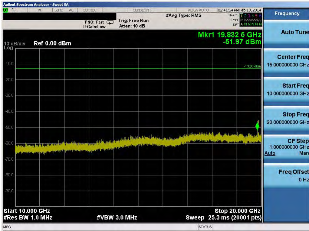
Plot 9-20. Conducted Spurious Plot (3.0MHz QPSK – RB Size 1, RB Offset 0 – Low Channel)
