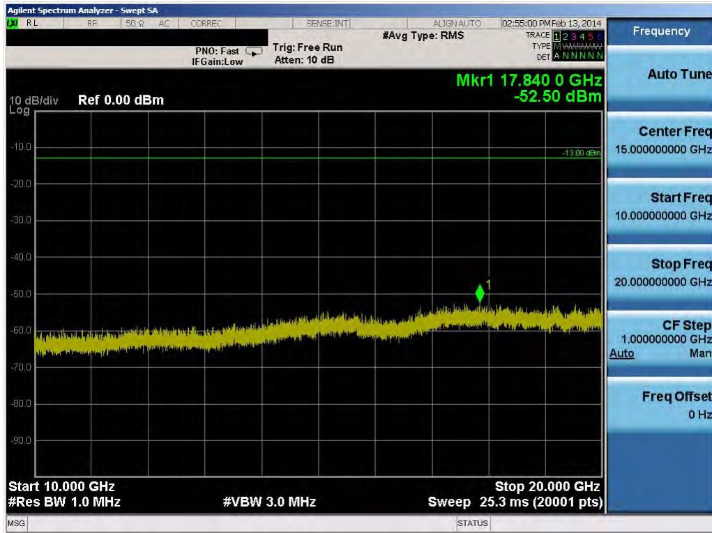
Plot 9-38. Conducted Spurious Plot (5.0MHz QPSK – RB Size 1, RB Offset 0 – High Channel)
