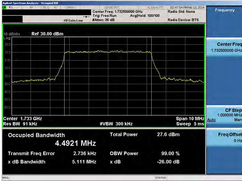
Plot 9-32. Occupied Bandwidth Plot (5.0MHz 16-QAM – RB Size 25)
