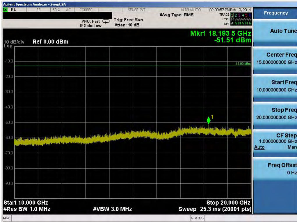
Plot 9-6. Conducted Spurious Plot (1.4MHz QPSK – RB Size 1, RB Offset 0 – Low Channel)
