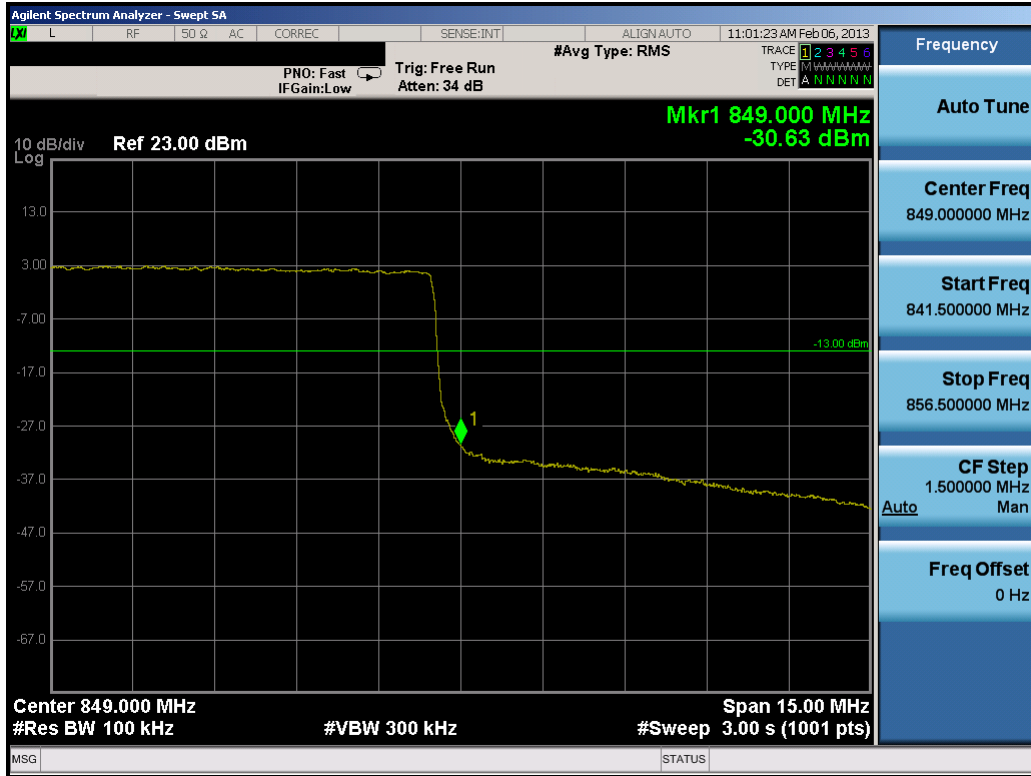
Plot 7-28. Upper Band Edge Plot (10.0MHz QPSK – RB Size 50)
