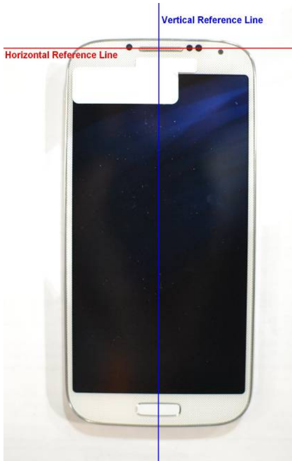
SAR Test Setup Photo 11 – DUT Reference lines
