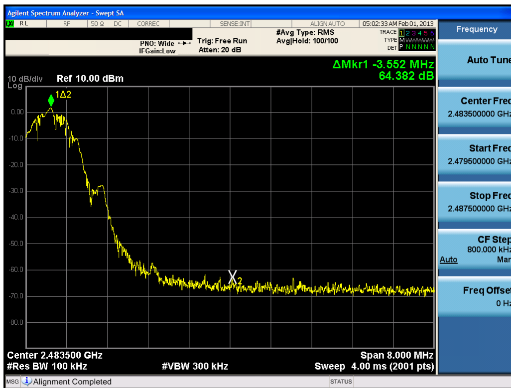
Plot 6-8. Band Edge Plot (Bluetooth (LE) – Ch. 39)
