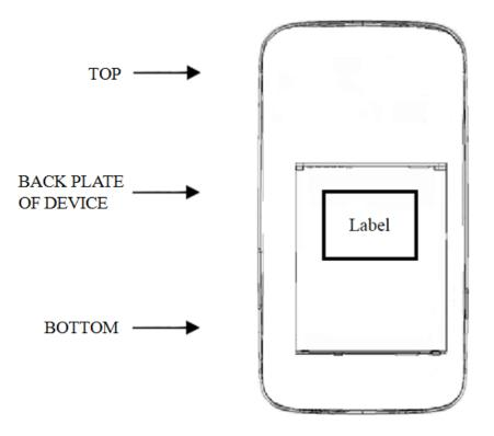
Phone : Label is placed inside of the battery compartment
