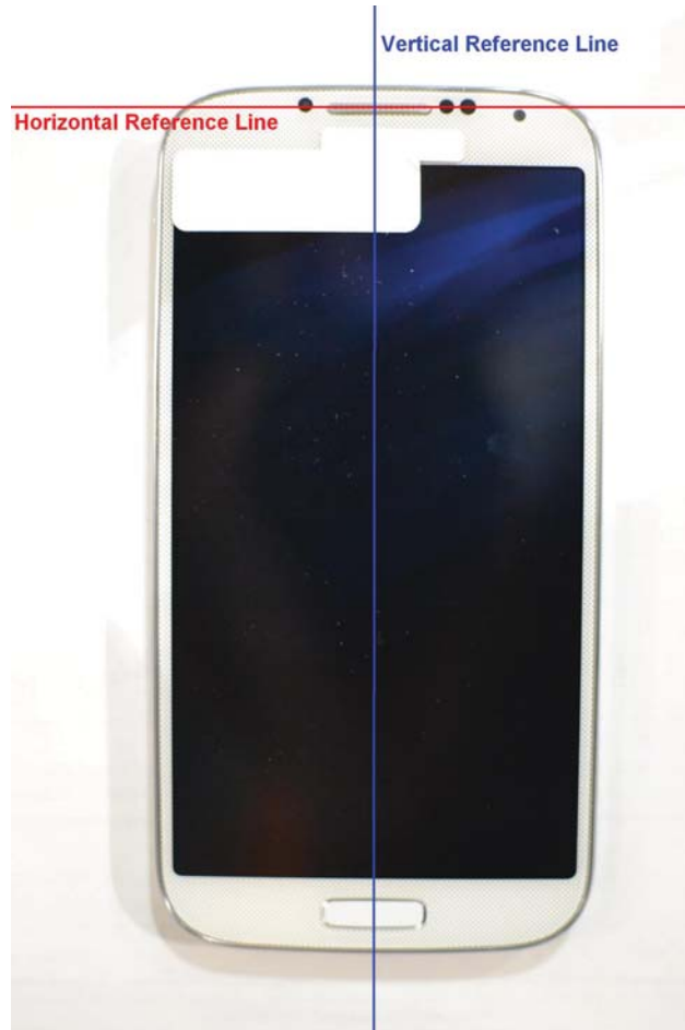
SAR Test Setup Photo 11 – Vertical and Horizontal Reference Lines
