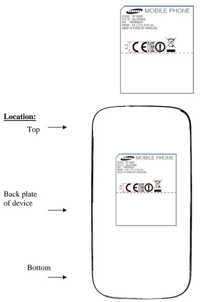
Label is placed inside of the battery compartment.
