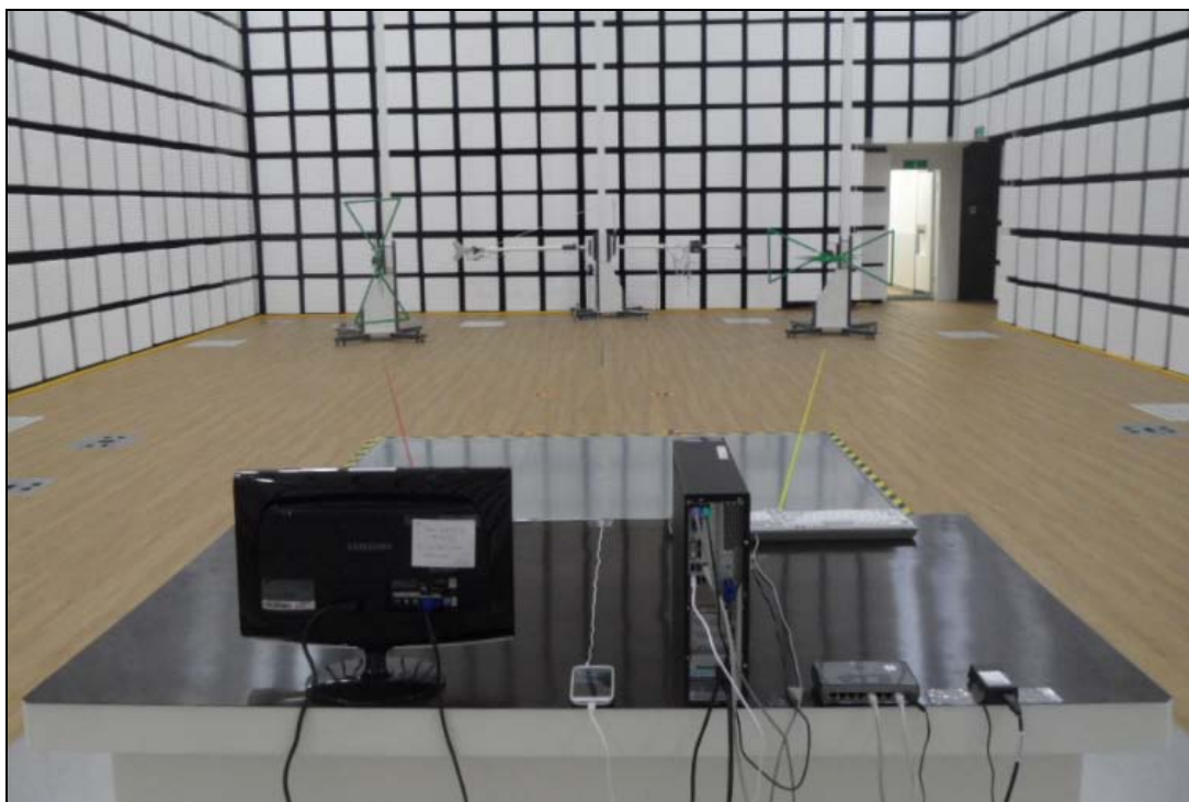
[ Radiated Disturbance for Below 1 GHz – Rear ]
