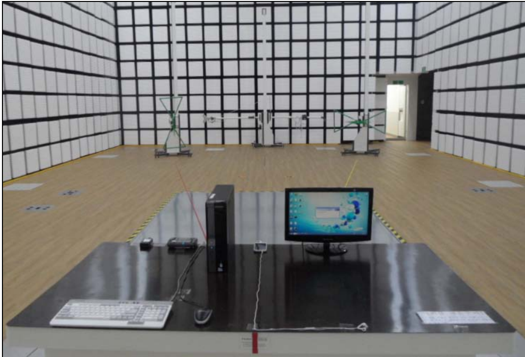
[ Radiated Disturbance for Below 1 GHz – Front ]
