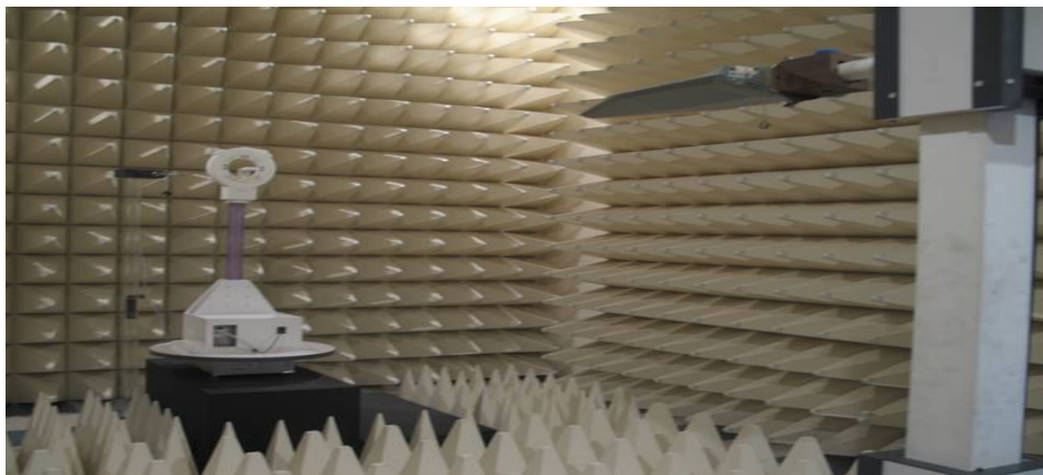
Figure2. Photograph of 3m Fully-Anechoic Chamber
