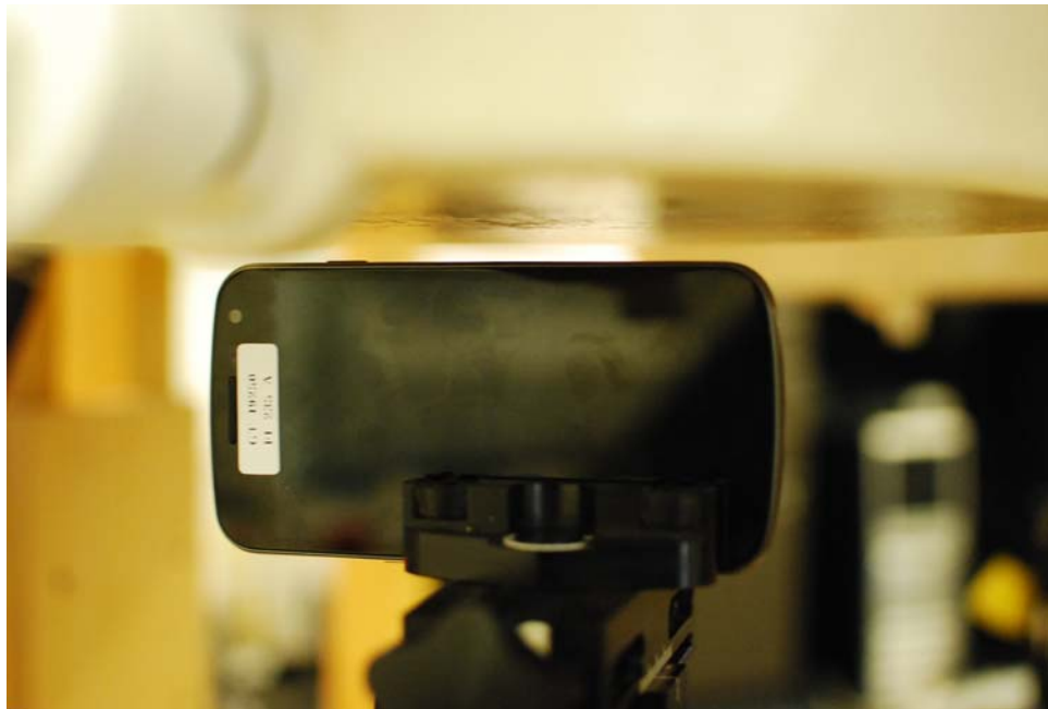
SAR Test Setup Photo 8: Right at 1.0 cm
