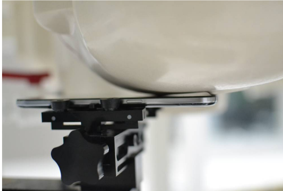
SAR Test Setup Photo 3 – Left Cheek
