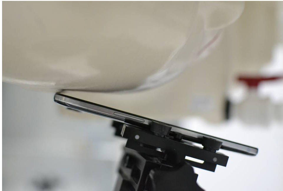
SAR Test Setup Photo 2 – Right Tilt
