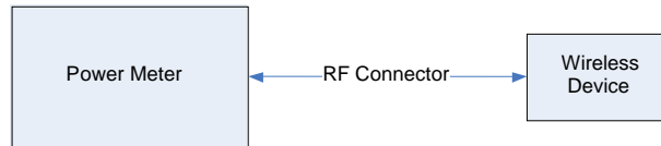
Figure 8-3 Power Measurement Setup
