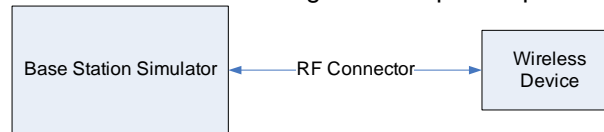
Figure 8-2 Power Measurement Setup
