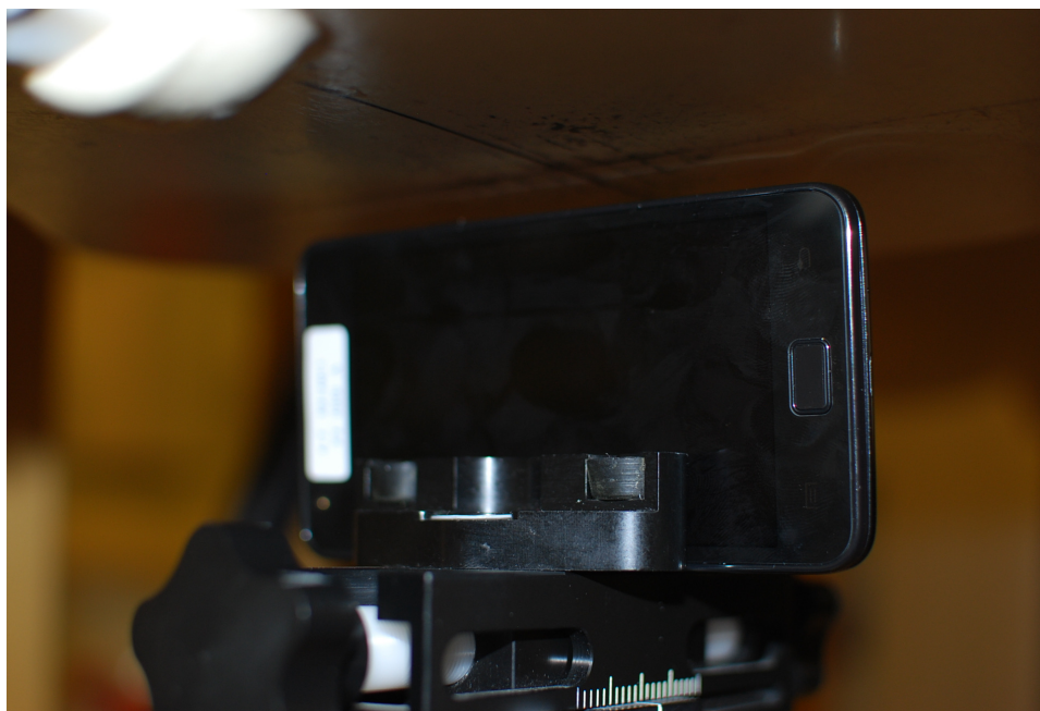
Figure 21-8 SAR Test Setup Photo 8: Right at 1.0 cm
