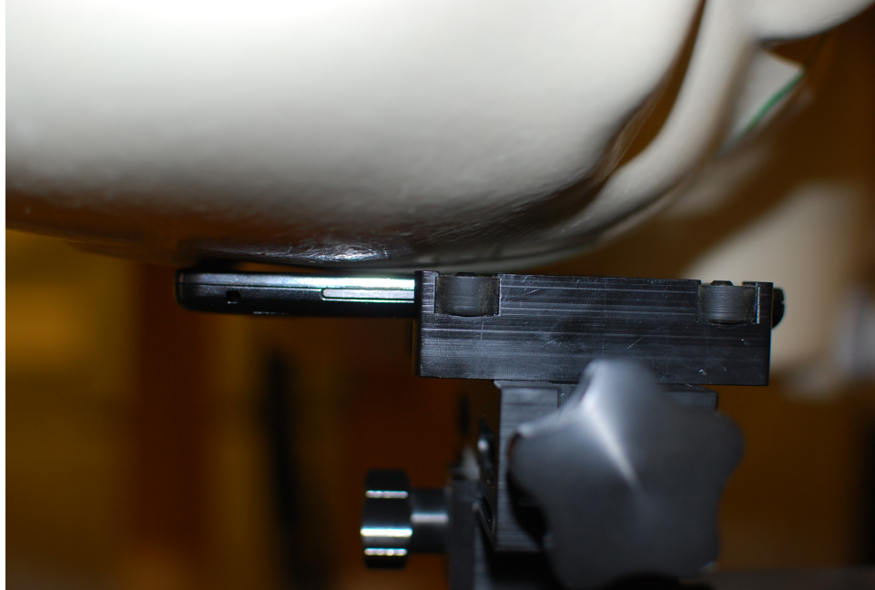
Figure 21-1 SAR Test Setup Photo 1: Right Touch
