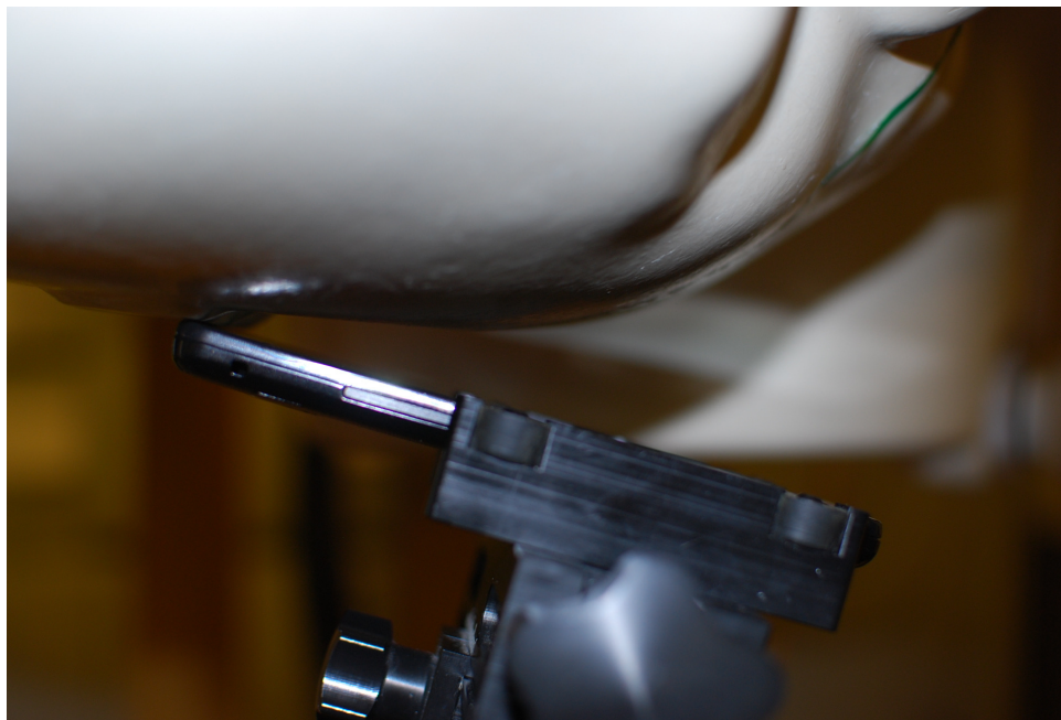
Figure 21-2 SAR Test Setup Photo 2: Right Tilt
