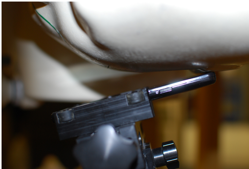
Figure 21-4 SAR Test Setup Photo 4: Left Tilt
