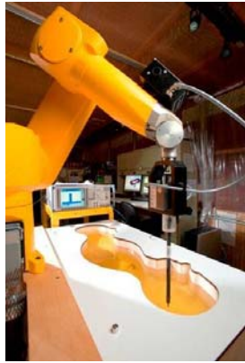
Figure 3-1 SAR Measurement System
