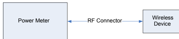
Figure 9-3 Power Measurement Setup
