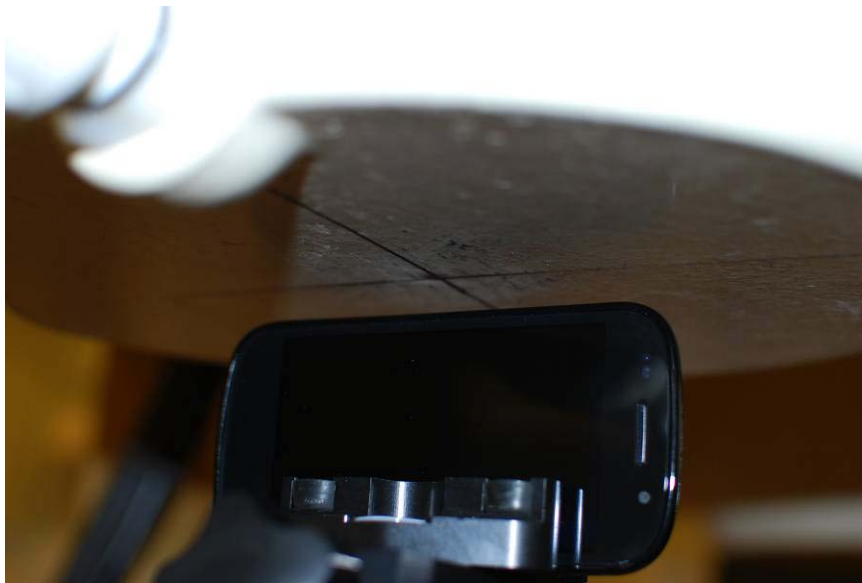
Figure 21-8 SAR Test Setup Photo – Left at 1.0 cm
