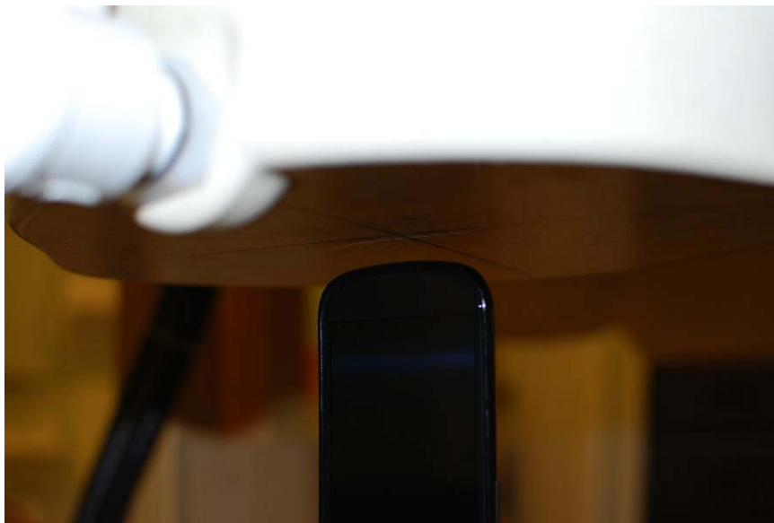
Figure 21-10 SAR Test Setup Photo – Bottom at 1.0 cm
