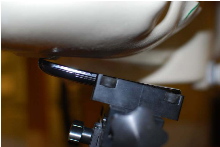
Figure 21-2 SAR Test Setup Photo – Right Tilt
