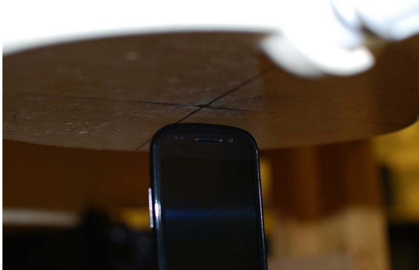
Figure 21-9 SAR Test Setup Photo – Top at 1.0 cm
