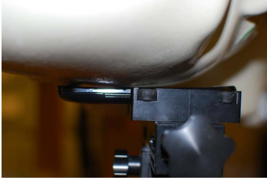
Figure 21-1 SAR Test Setup Photo – Right Touch
