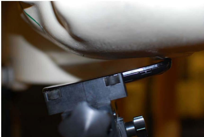
Figure 21-4 SAR Test Setup Photo – Left Tilt
