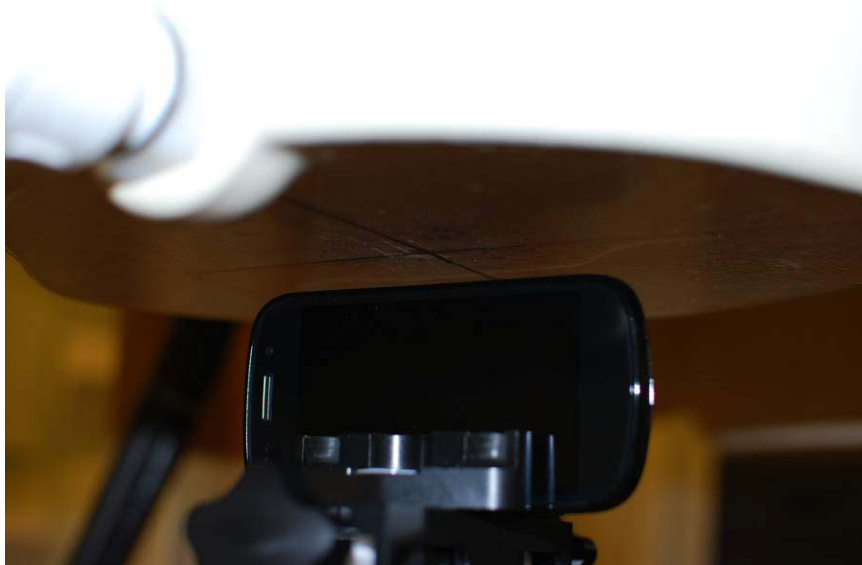
Figure 21-7 SAR Test Setup Photo - Right at 1.0 cm
