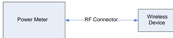
Figure 12-1 Power Measurement Setup
