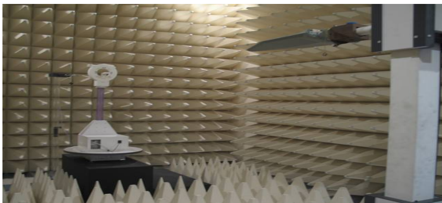
Figure2. Photograph of 3m Fully-Anechoic Chamber
