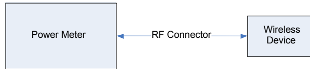
Figure 14-2 Power Measurement Setup
