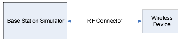
Figure 14-1 Power Measurement Setup
