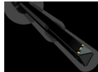
Figure 4-3 Triangular Probe Configuration
