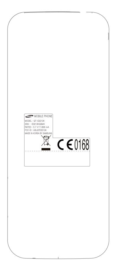
Note: The FCC ID label shown will be readily visible at the time of purchase. The label is placed inside the battery compartment
