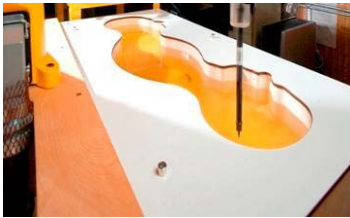
Figure 6-2 SAM Phantom with Simulating Tissue
