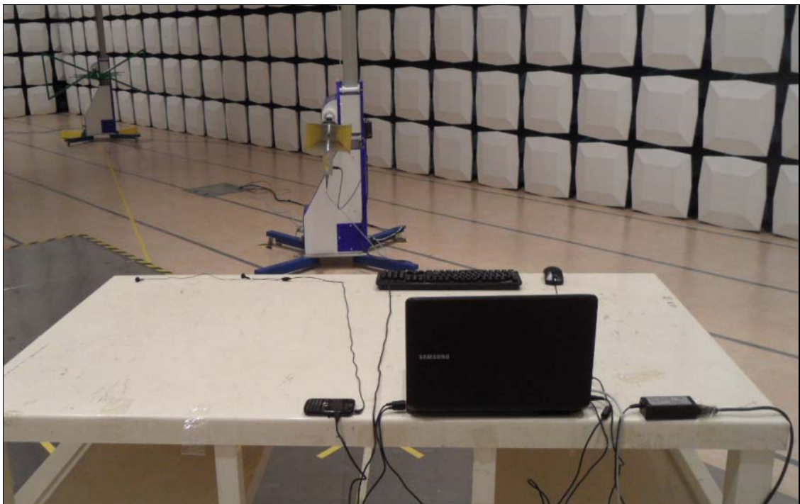
[ Radiated Disturbance for Above 1 GHz – Rear ]
