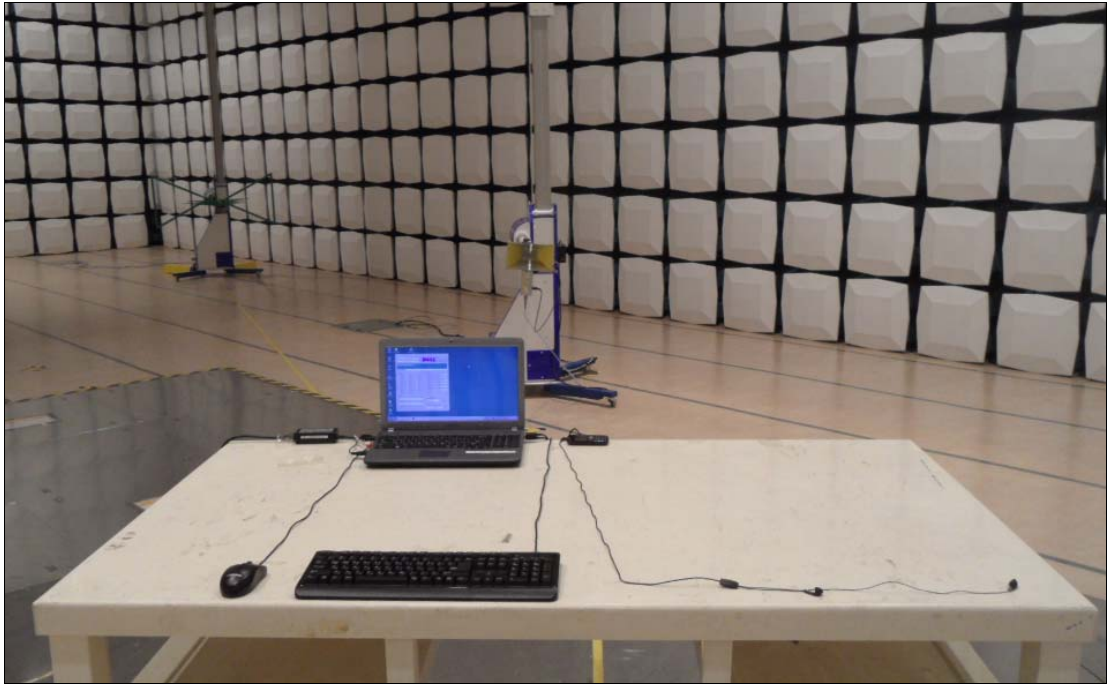
[ Radiated Disturbance for Above 1 GHz – Front ]
