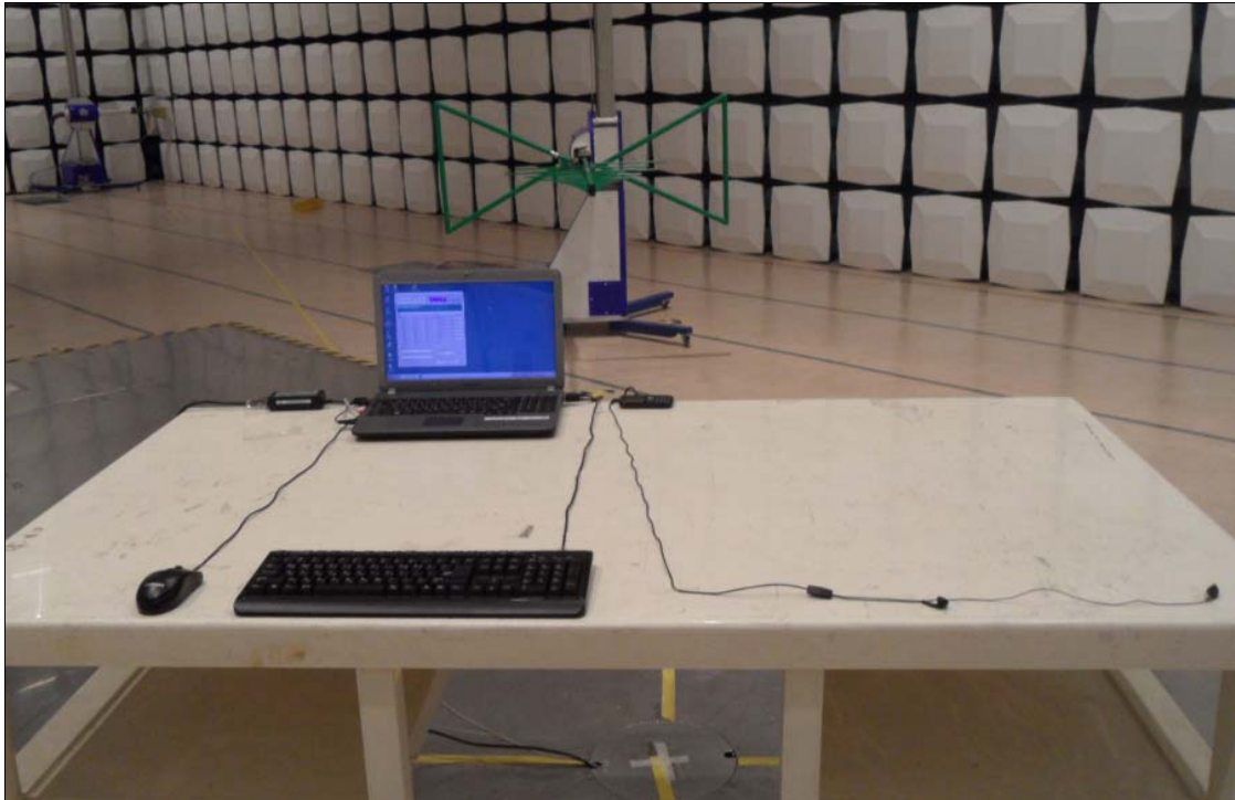
[ Radiated Disturbance for Below 1 GHz – Front ]
