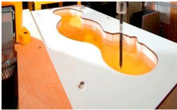
Figure 6-2 SAM Phantom with Simulating Tissue
