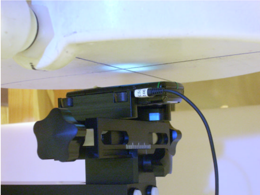
Figure 13: Body SAR, Front Side with 15mm Space
