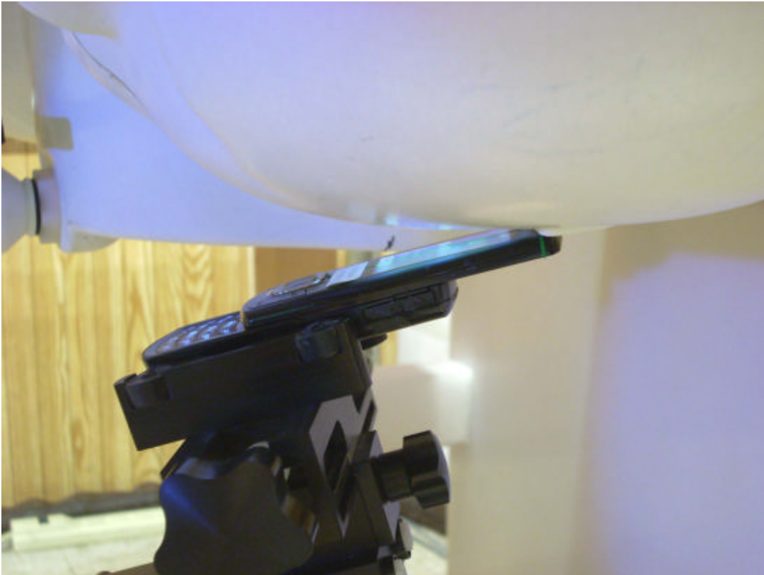
Figure 10: Left Head SAR, 15° Tilt, Slide Out
