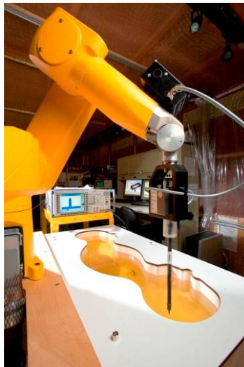
Figure 3-2 DASY4 SAR Measurement System
